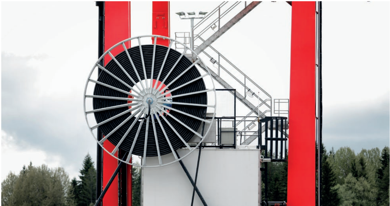
RTG electrification options are cable reel and bus bar.
