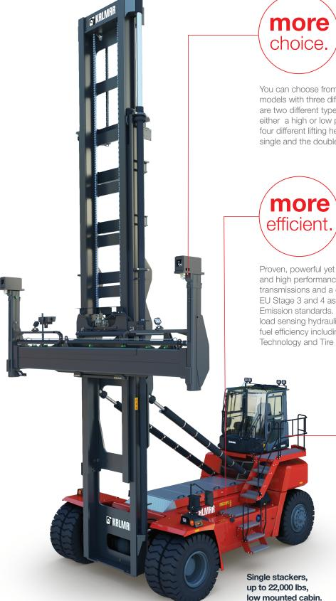
You can choose from either a single or double stacker models with three different lifting capacities each. There are two different types of cabins that can be mounted in either a high or low position, four spreader options and four different lifting heights to choose from for both the single and the double stackers.
