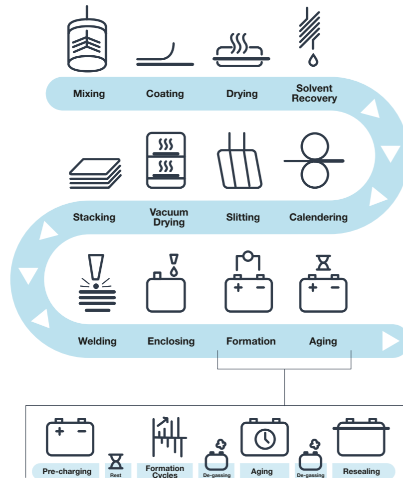
Schematic of LIB manufacturing processes Source: Sciencedirect
